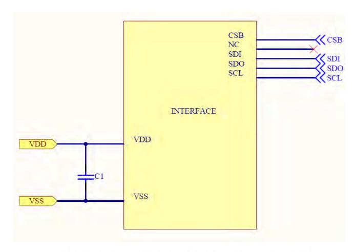
Pin connected to MCU interface: CSB, SDI,SDO, SCL
