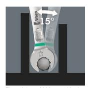
6003 combination The Joker wrench with its special mouth geometry - an open-end offset by 7.5° and the double hexagon geometry - doubles the placement possibilities when repeatedly turning the wrench 180° around the longitudinal axis. Bolts and screw heads can be "accessed" every 15°. The Joker 6003 will automatically find the respective placement point after every turn.
