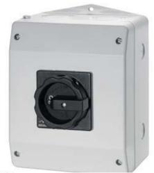
MAIN SWITCH 6-POLE IU=25, P/AC-23A AT 400V=9,5KW 1NO+1NC, 1 N-TERMINAL MOULDED-PLASTIC ENCLOSURED, IP65
