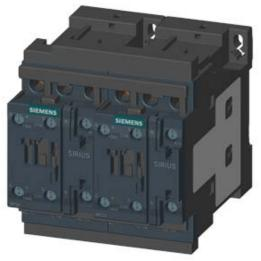
REV. COMB., AC3, 5.5KW/ 400V DC24V 3-POLE, SZ S0 SCREW TERMINAL ELECTR. AND MECH. INTERLOCK 2NO INTEGR.
