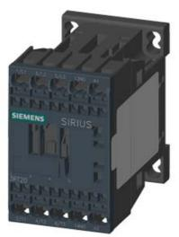
CONTACTOR, AC-3, 5.5KW/400V, 1NO, AC 230V, 50/60 HZ, 3-POLE, SZ S00 SPRING-LOADED TERMINAL
