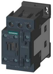
CONTACTOR, AC-3, 5.5KW/400V, 1NO+1NC, AC 48V 50HZ, 3-POLE, SZ S0 SCREW TERMINAL
