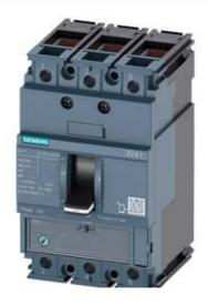
CIRCUIT BREAKER 3VA1 IEC FRAME 160 BREAKING CAPACITY CLASS S ICU=36KA @ 415 V 3-POLE, LINE PROTECTION TM220, ATFM, IN=50A OVERLOAD PROTECTION IR=35A ...50A SHORT CIRCUIT PROTECTION II=10 X IN CABLE CONNECTION
