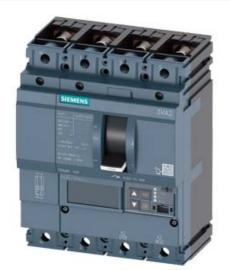
CIRCUIT BREAKER 3VA2 IEC FRAME 100 BREAKING CAPACITY CLASS C ICU=110KA @ 415 V 4POLE, LINE PROTECTION ETU850, LSI, IN=40A OVERLOAD PROTECTION IR=16A ...40A SHORT CIRCUIT PROTECTION ISD=0,6..10X IN, II=1,5..12X IN NEUTRAL PROTECTION ADJUSTABLE (OFF, UPTO 160%) BUSBAR CONNECTION
