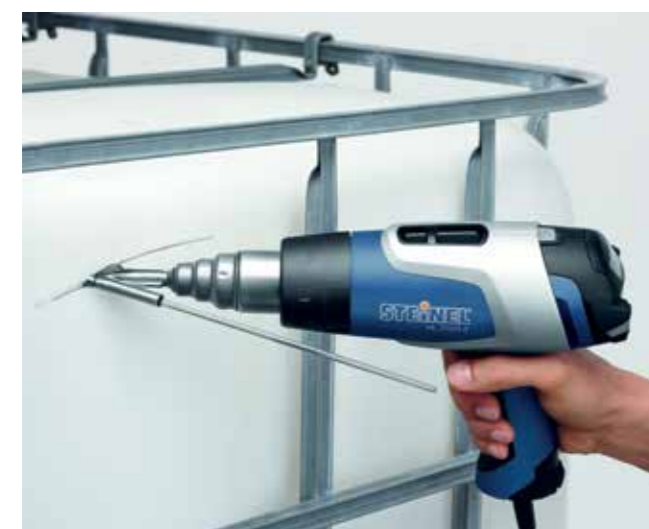
Repairing. Welding PVC water tank.
