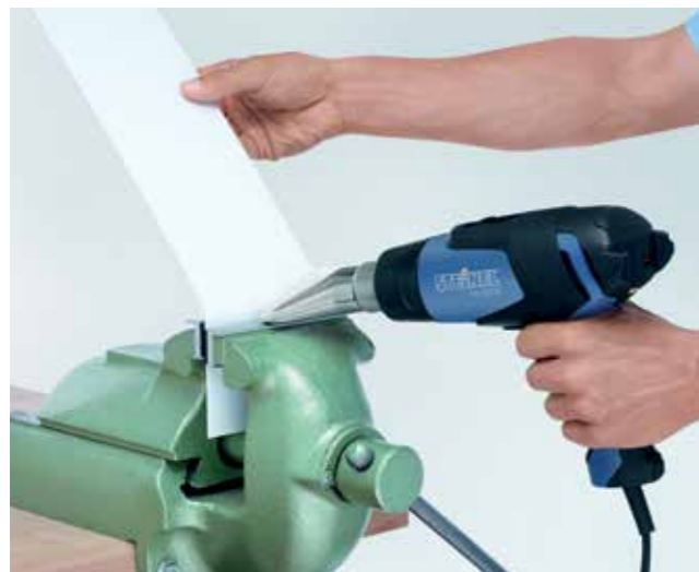
Shaping. Using heat for getting plastic into exactly the right shape.
