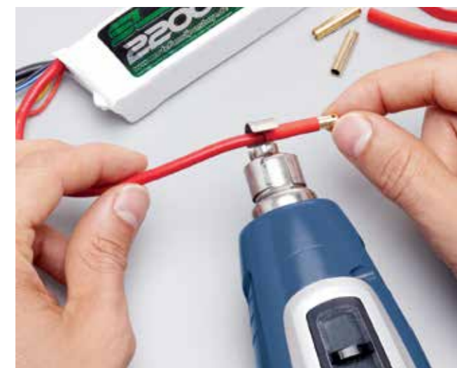
Heat-shrinking. Secure standing for hands-free work.
