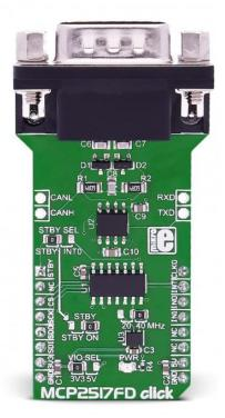
Note: For selecting the interface voltage level, use the onboard jumper, and choose between the 3.3V and 5V. For more information, see the Jumpers and Settings table below.
