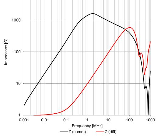
CHECKED REVISION DATE (YYYY-MM-DD) GENERAL TOLERANCE PROJECTION METHOD HasA 001.001 2021-01-08 DIN ISO 2768-1m **WE-CMB HC Common Mode** Würth Elektronik eiSos GmbH & Co. KG **Power Line Choke** ORDER CODE EMC & Inductive Solutions Max-Eyth-Str. 1 7448226404 74638 Waldenburg SIZE/TYPE STATUS Tel. +49 (0) 79 42 945 - 0 BUSINESS UNIT PAGE www.we-online.com Valid 2/6 Type S eiSos eiSos@we-online.com
