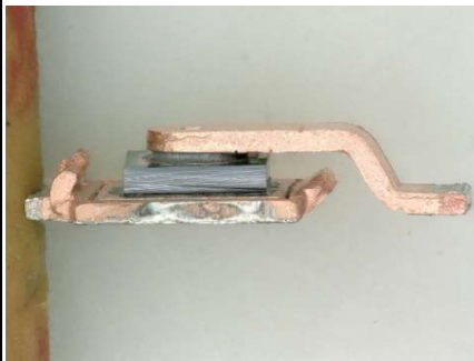
Sub-assembly (Side view)
