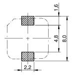
no sensitive traces underneath the component
