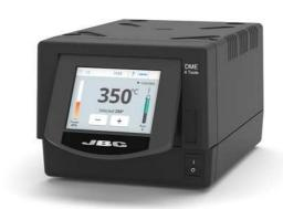
This control unit operates with **four tools simultaneously for soldering or desoldering tools** and is fully compatible with 10 different JBC Tools delivering up to 160 W per tool.
