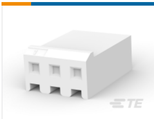
TE Part #1-647402-5 3.96mm Wire-to-board housing: receptacle, with mating alignment, SL 156
