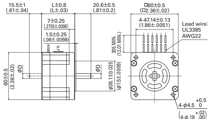
Note: A unipolar motor is illustrated; bipolar motors have four lead wires.
