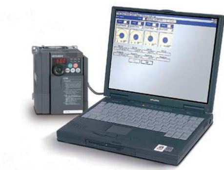
Configuring the drive via a Windows laptop
