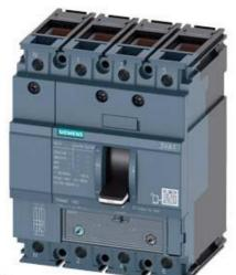
CIRCUIT BREAKER 3VA1 IEC FRAME 160 BREAKING CAPACITY CLASS S ICU=36KA @ 415 V 4-POLE, LINE PROTECTION TM240, ATAM, IN=20A OVERLOAD PROTECTION IR=14A ...20A SHORT CIRCUIT PROTECTION II=5...10 X IN NEUTRAL UNPROTECTED CABLE CONNECTION
