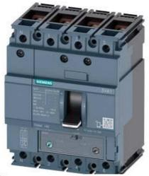
CIRCUIT BREAKER 3VA1 IEC FRAME 160 BREAKING CAPACITY CLASS H ICU=70KA @ 415 V 4-POLE, LINE PROTECTION TM240, ATAM, IN=50A OVERLOAD PROTECTION IR=35A ...50A SHORT CIRCUIT PROTECTION II=5...10 X IN NEUTRAL UNPROTECTED BUSBAR CONNECTION
