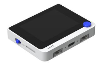
Wio Terminal is a perfect tool to get started with IoT and TinyML – it is built around ATSAMD51P19 chip with ARM Cortex–M4F core running at 120MHz, which is very well supported by various frameworks for ML inference on microcontrollers.
