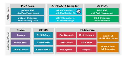
MDK-Core is based on μVision with leading support for Cortex-M devices while DS-MDK contains the Eclipse-based DS-5 IDE/Debugger and supports 32-bit Cortex-A processors or hybrid systems with 32-bit Cortex-A and Cortex-M.
