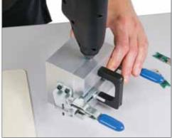
Securely close the mould shut with the component inside. Place the nozzle of the applicator into the injection hole in the side of the aluminium mould, and dispense the liquid resin, fill the mould as quickly as possible and maintain trigger pressure for 5-15 seconds, after filling to reduce shrinkage.
