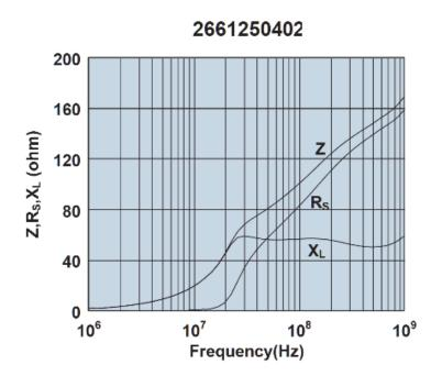
Impedance, reactance, and resistance vs. frequency.
