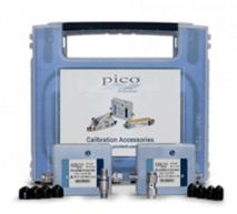
PicoVNA Dual E-Cal 8.5 GHz Automated calibration kit (SMA)
