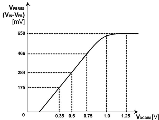
Figure 24. LED Current De-rating Function (DC Dimming Function)
