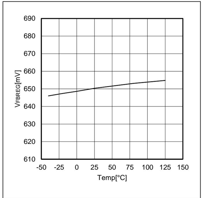
Figure 6. VFBREG vs Temp
