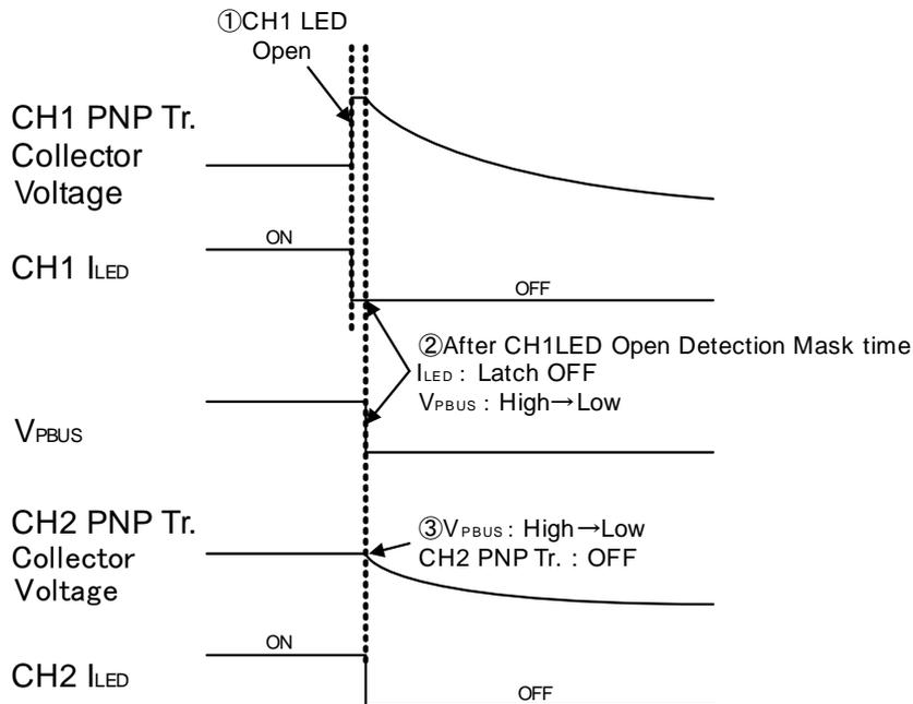
Figure 26. Example of Protective Operation
