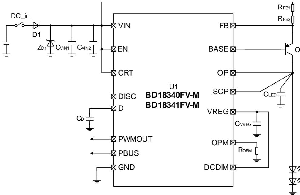
Figure 29. Recommended Application Circuit1 (I<sub>LED</sub> 120mA, LED white 2strings)
