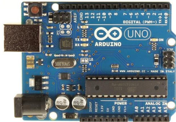
The Uno differs from all preceding boards in that it does not use the FTDI USB-to-serial driver chip. Instead, it features the Atmega16U2 (Atmega8U2 up to version R2) programmed as a USB-to-serial converter.
