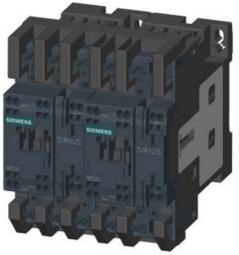
REV. COMB., AC3, 18.5KW/ 400V DC24V 3-POLE, SZ S0 SPRING-LOADED TERMINAL ELECTR. AND MECH. INTERLOCK 2NO INTEGR.
