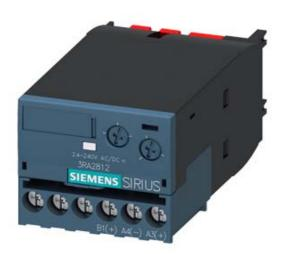
SOLID-STATE TIME RELAY OFF-DELAY WITH AUXILIARY VOLTAGE AND SEMICONDUCTOR OUTPUT 24...240V AC/DC TIME RANGE 0.05...100S FOR SNAPPING ONTO THE FRONT; FOR 3RT2 CONTACTORS S00/S0 SCREW TERMINALS INTEGRATED VARISTOR FOR DAMPING CONTACTOR COILS
