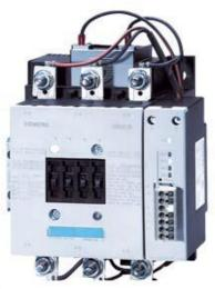
CONTACTOR, 75KW/400V/AC-3 AC(40...60HZ)/DC OPERATION UC 96-127V AUXILIARY CONTACTS 1NO+1NC 3-POLE, SIZE S6 BAR CONNECTIONS ELECTRONIC OPERATING MECHANISM WITH PLC/SIMOCODE INTERFACE AND REMAIN. LIFETIME INDICATOR
