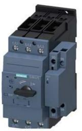
CIRCUIT BREAKER, SIZE S2, FOR MOTOR PROTECTION, CLASS 10, W. OVERLOAD RELAY FUNCTION A-RELEASE 35...45A, N-RELEASE 650A, STANDARD BREAKING CAPACITY
