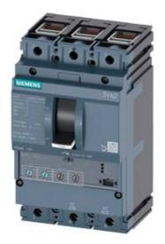
CIRCUIT BREAKER 3VA2 IEC FRAME 100 BREAKING CAPACITY CLASS M ICU=55KA @ 415 V 3POLE, LINE PROTECTION ETU350, LSI, IN=40A OVERLOAD PROTECTION IR=16A ...40A SHORT CIRCUIT PROTECTION ISD=1,5... 10 X IR, II=12 X IN CABLE CONNECTION
