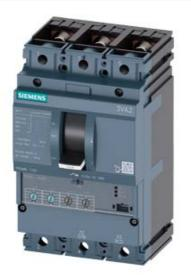
CIRCUIT BREAKER 3VA2 IEC FRAME 100 BREAKING CAPACITY CLASS H ICU=85KA @ 415 V 3POLE, LINE PROTECTION ETU350, LSI, IN=40A OVERLOAD PROTECTION IR=16A ...40A SHORT CIRCUIT PROTECTION ISD=1,5... 10 X IR, II=12 X IN BUSBAR CONNECTION
