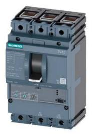
CIRCUIT BREAKER 3VA2 IEC FRAME 160 BREAKING CAPACITY CLASS C ICU=110KA @ 415 V 3POLE, LINE PROTECTION ETU320, LI, IN=160A OVERLOAD PROTECTION IR=64A ...160A SHORT CIRCUIT PROTECTION II=10 X IN CABLE CONNECTION
