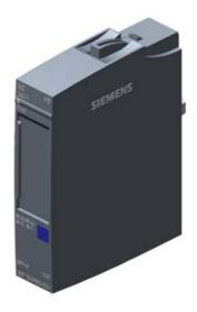
SIMATIC ET 200SP, ANALOG OUTPUT MODULE, AQ 2 X U/I HIGH SPEED, FITS TO BU-TYPE A0, A1, COLOR CODE CC00, CHANNEL DIAGNOSIS, 16BIT, +/-0,3%
