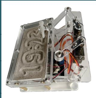
The Raspberry Pi Pico Sandclock kit is an innovative mix of technology and design. It allows you to build a sandclock that uses servo motors to write the time in sand and then erases it with vibration motors. Made from clear acrylic components, this kit offers a fascinating insight into the mechanics of time representation. Easy to assemble and ideal for technology enthusiasts, this kit is a perfect example of the combination of creative timekeeping and modern technology.
