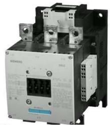
CONTACTOR, 160KW/400V/AC-3 AC(40...60HZ)/DC OPERATION UC 110-127V AUXILIARY CONTACTS 2NO+2NC 3-POLE, SIZE S10 BAR CONNECTIONS CONVENT. OPERATING MECHANISM CAGE CLAMP TERMINAL
