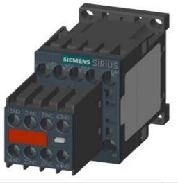
CONTACTOR, AC-3, 5.5KW/400V, 2NO+2NC, AC 230V, 50/60 HZ, 3-POLE, SZ S00 SCREW TERMINAL PERMANENT AUX. SWITCH FOR SUVA APPLICATIONS
