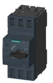
CIRCUIT-BREAKER SZ S00, FOR STARTER COMBINATION, RATED CURRENT 8A, N-RELEASE 104A, SPRING-L. CONNECTION, STANDARD SW. CAPACITY
