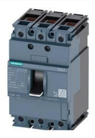
CIRCUIT BREAKER 3VA1 IEC FRAME 160 BREAKING CAPACITY CLASS S ICU=36KA @ 415 V 3-POLE, LINE PROTECTION TM210, FTFM, IN=16A OVERLOAD PROTECTION IR=16A FIXED SHORT CIRCUIT PROTECTION II=20 X IN CABLE CONNECTION
