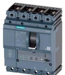
CIRCUIT BREAKER 3VA2 IEC FRAME 100 BREAKING CAPACITY CLASS L ICU=150KA @ 415 V 4POLE, LINE PROTECTION ETU330, LIG, IN=100A OVERLOAD PROTECTION IR=40A ...100A SHORT CIRCUIT PROTECTION II=1,5...12 X IN NEUTRAL PROTECTION ADJUSTABLE(OFF,50%,100%) GROUNDFAULTPROTECTION IG=0,2... 1 X IN, TG=0,1/0,3MS BUSBAR CONNECTION
