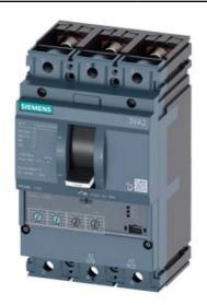
CIRCUIT BREAKER 3VA2 IEC FRAME 100 BREAKING CAPACITY CLASS M ICU=55KA @ 415 V 3POLE, LINE PROTECTION ETU330, LIG, IN=63A OVERLOAD PROTECTION IR=25A ...63A SHORT CIRCUIT PROTECTION II=1,5...12 X IN GROUNDFAULTPROTECTION IG=0,2... 1 X IN, TG=0,1/0,3MS BUSBAR CONNECTION
