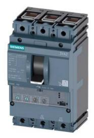
CIRCUIT BREAKER 3VA2 IEC FRAME 160 BREAKING CAPACITY CLASS C ICU=110KA @ 415 V 3POLE, LINE PROTECTION ETU350, LSI, IN=25A OVERLOAD PROTECTION IR=10A ...25A SHORT CIRCUIT PROTECTION ISD=1,5... 10 X IR, II=12 X IN CABLE CONNECTION
