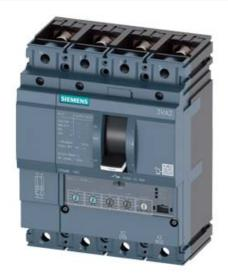
CIRCUIT BREAKER 3VA2 IEC FRAME 160 BREAKING CAPACITY CLASS C ICU=110KA @ 415 V 4POLE, LINE PROTECTION ETU350, LSI, IN=63A OVERLOAD PROTECTION IR=25A ...63A SHORT CIRCUIT PROTECTION ISD=1,5... 10 X IR, II=12 X IN NEUTRAL PROTECTION ADJUSTABLE(OFF,100%) BUSBAR CONNECTION
