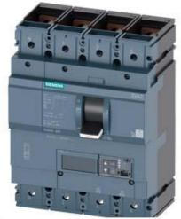
CIRCUIT BREAKER 3VA2 IEC FRAME 400 BREAKING CAPACITY CLASS H ICU=85KA @ 415 V 4-POLE, LINE PROTECTION ETU850, LSI, IN=400A OVERLOAD PROTECTION IR=160A ...400A SHORT CIRCUIT PROTECTION ISD=0,6..10X IN, II=1,5..10X IN NEUTRAL PROTECTION ADJUSTABLE (OFF, UPTO 100%) BUSBAR CONNECTION
