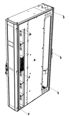
Fig. 40: Attach the brackets to the LCP
