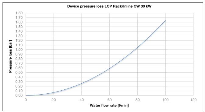
Fig. 124: Pressure loss of the LCP CW in the "30 kW" version
