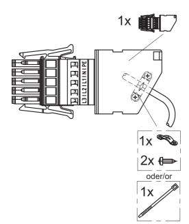
Fig. 71: Schematic diagram of the connector with three-phase connection – global version
