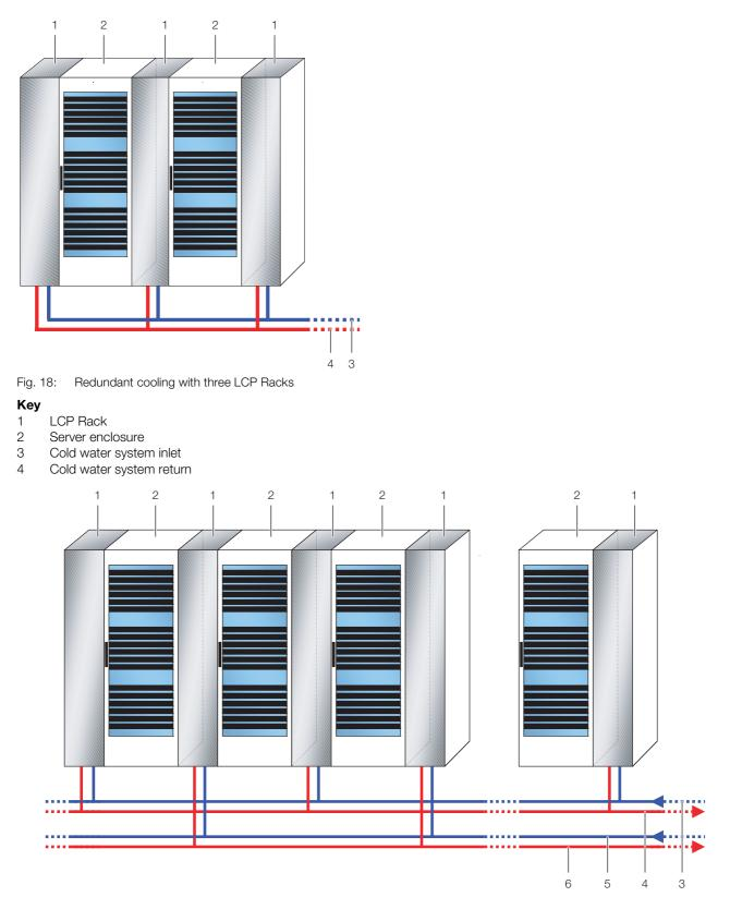
Fig. 19: Redundant cooling and double alternating water supply
