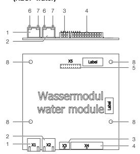
Fig. 132: Control unit water module - rear/top view
