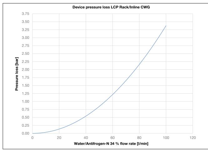
Fig. 125: Pressure loss of the LCP CWG
