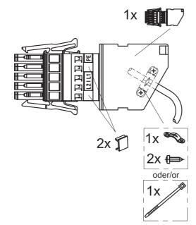
Fig. 77: Connector diagram for single-phase connection – NSA version
