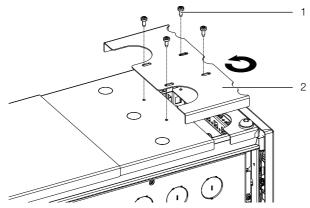
Fig. 81: Rotate the roof plate
