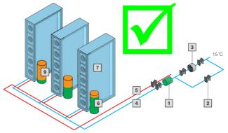
Fig. 86: Cooling distribution with Tichelmann principle
