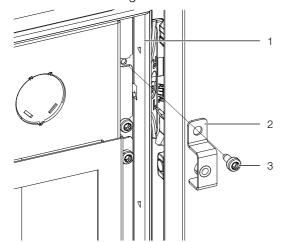
Fig. 39: Mounting bracket for attaching the side panel
