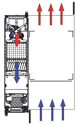
If the need arises, both the front and the rear door are automatically opened. The air flows unhindered into the interior of the enclosure, circulates around the installed equipment and exits the system via the open rear door of the enclosure. It is important to ensure that the LCP fans are switched off, otherwise hot air will be blasted in front of the 482.6 mm (19") level in the event of emergency cooling.
