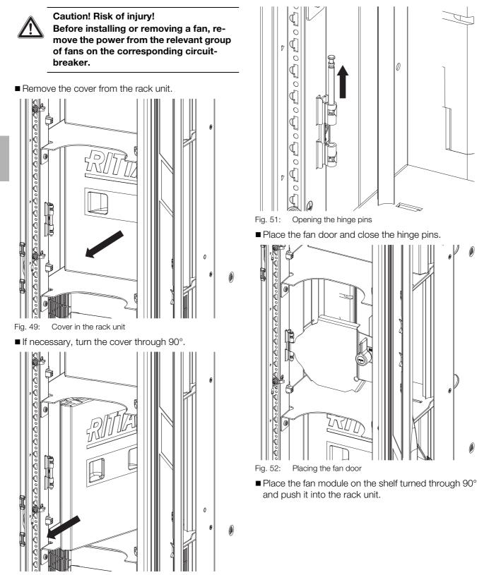
Fig. 50: Turned cover in the rack unit
