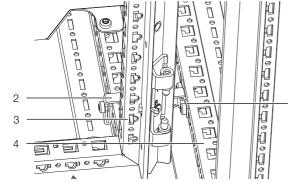
Fig. 35: Connection element in the rear area VX/VX
