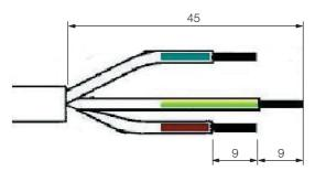
Fig. 75: Dimensions for removing the rubber sheathing and insulation
