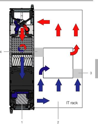
Fig. 29: Placement of foam strips for devices with sideways air throughput (top view) – LCP Rack
