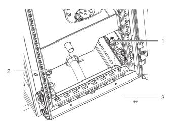
Fig. 21: Transport brace (2 x screws)
