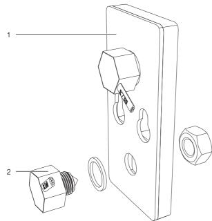
Fig. 67: Fastening the level sensor
