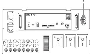
Fig. 57: Connection point at the electronic module
