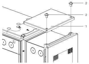
Fig. 33: Mounting the adaptor frame roof plate
