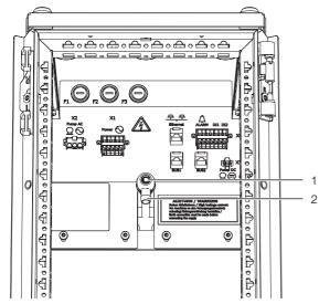
Fig. 88: Bleeding the air from the heat exchanger
