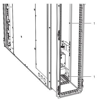
Fig. 32: Mounting the adaptor frame
