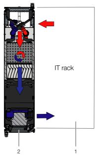
Fig. 134: "Front to back" cooling principle with bayed LCP Rack
