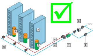
Fig. 85: Cooling distribution with hydraulic balancing
