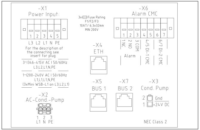
Fig. 128: Wiring diagram global version
