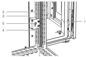
Fig. 38: Bracket and screws in the front area VX/TS
