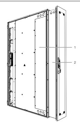
Fig. 31: Adaptor on the LCP Inline
