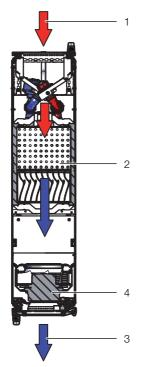
Fig. 3: Air routing on the LCP Inline Flush - top view
