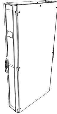
Fig. 42: Fitted side panel
