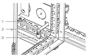
Fig. 36: Connection element in the rear area VX/TS
