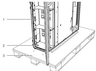
Fig. 20: Front fastening (2 x screws)
