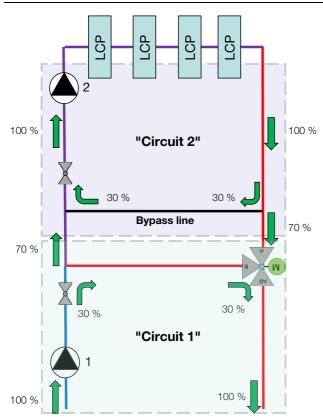
Fig. 83: Injection circuit (layout diagram)
