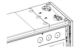
Fig. 82: Rotated roof plate
