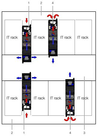
Fig. 27: Installation room with cold aisle compartmentalisation **Key**
