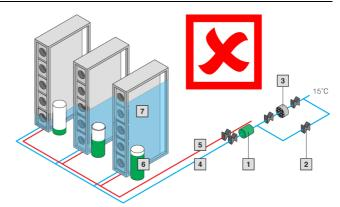
Fig. 84: Cooling distribution without hydraulic balancing
