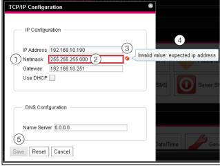
Fig. 110: Display of an incorrect entry
