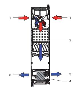
Fig. 1: Air routing on the LCP Rack - top view
