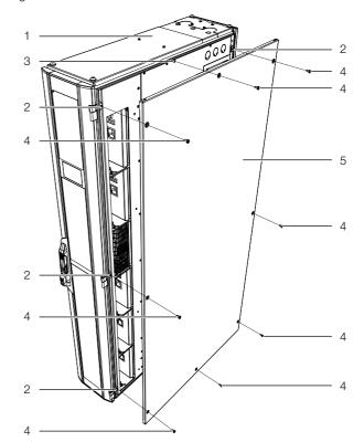
Fig. 41: Attach the side panel to the LCP
