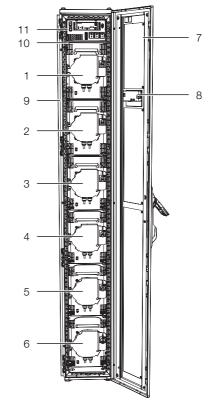
Fig. 13: Liquid Cooling Package front – open front door
