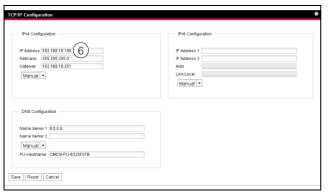
Fig. 91: Adjusting the TCP/IP settings
