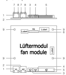
Fig. 131: Control unit fan module - rear/top view
