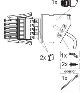
Fig. 78: Connector diagram for two-phase connection – NSA version
