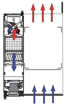
Perforated server rack front door in conjunction with a glass or sheet steel enclosure rear door
