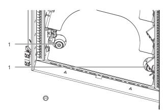
Fig. 23: Remove the transport brace screws
