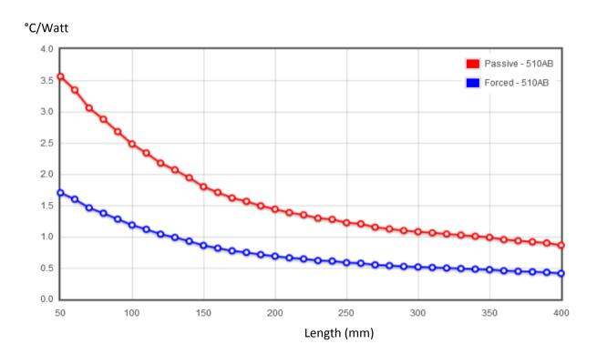
Thermal Resistance is calculated based on a distributed heat load and vertically mounted fins anodised heatsink with a 60°C temperature.
