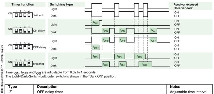
Time  $t_{ON}$ ,  $t_{OFF}$  and  $t_{OS}$  are adjustable from 0.02 to 1 seconds. The Light-/Dark-Switch (Left, outer switch) is shown in the "Dark ON" position.
