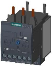
OVERLOAD RELAY 6...25 A FOR MOTOR PROTECTION SIZE S0, CLASS 5...30 CONTACTOR ASS. MAIN CIRCUIT: SCREW CONN. AUX.CIRCUIT: SCREW CONN. MANUAL-AUTOM.-RESET INT. GROUND FAULT DETECTION
