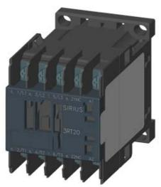
CONTACTOR, AC-3, 4KW/400V, 1NC, AC 100V 50HZ, 100...110V 60HZ 3-POLE, SZ S00 RING CABLE LUG CONNECTION
