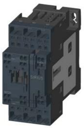
CONTACTOR, AC-3, 7.5KW/400V, 1NO+1NC, DC 24V, COM. CAPABILITY, 3-POLE, SZ S0 SPRING-LOADED TERMINAL
